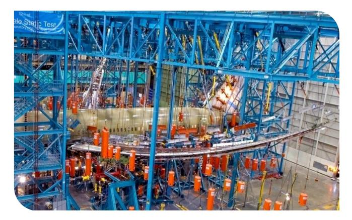
Full scale structural test of Boeing 787 ODiSI used to measure strain distribution in composite materials
