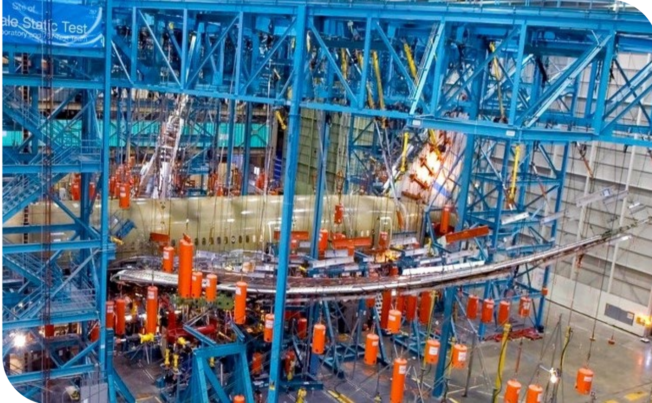
Full scale structural test of Boeing 787 ODiSI used to measure strain distribution in composite materials
